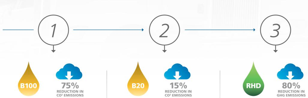
**Pure biodiesel, known as B100,** reduces carbon dioxide emissions by more than **75 percent** compared with petroleum diesel, according to the U.S. government.<sup>7</sup>
